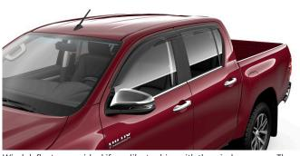
Wind deflectors are ideal if you like to drive with the windows open. They are custom designed to match the aerodynamic contours of your vehicle and work by diverting air flow to ensure that you and your passengers are not troubled by excessive wind movement and noise.
