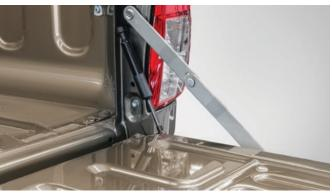
Tailgate struts are essential for the suspension of your tailgate. The strut helps facilitate closing the tailgate by assisting in pulling it upwards once you start to push/pull it upwards.
