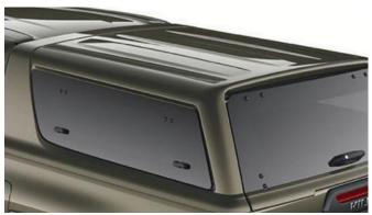
The Hilux leisure hardtop features a double shell plastic ABS canopy for extra robustness with lockable, hinged and tinted pop out windows and interior battery powered LED lights. \*Available in a selection of colours. \*NA For GR Sport
